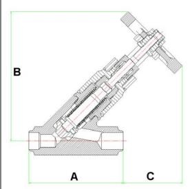
Seal Welded Bonnet Valve - Oblique Pattern. Standard Bore, Outside Screw and Yoke, Non-rising handwheel, Seal Welded Bonnet.
